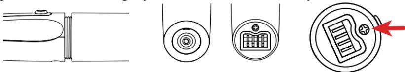
Figure 9 Replacement of battery
